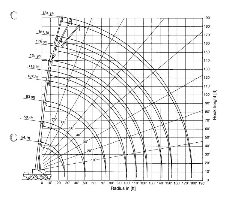
**NOTE**: Load Radius is measured in feet from Axis of Rotation. Boom and jib geometry shown are for unloaded condition and machine standing level on firm supporting surface. Boom deflection and subsequent radius and boom angle change must be accounted for when applying load to hook.
